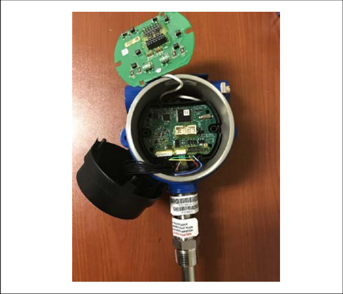
Fig. 11: Top Board Removed
