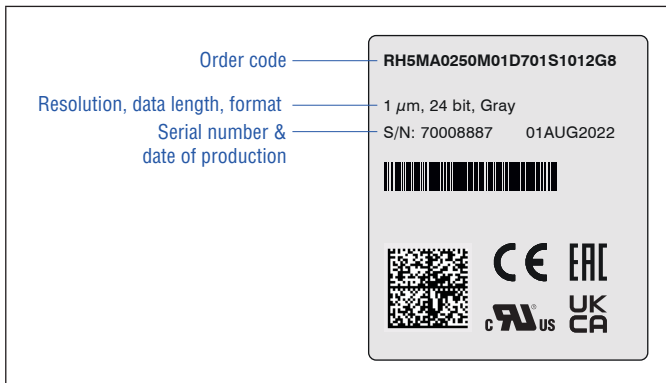
Fig. 1: Example of nameplate of R-Series V RH5 sensor with SSI output
