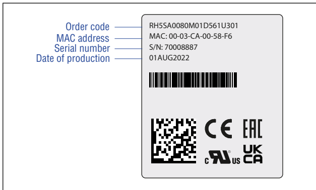
Fig. 1: Example of nameplate of R-Series V RH5 sensor with POWERLINK output
