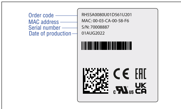
Fig. 1: Example of nameplate of a R-Series V RH5 sensor with EtherNet/IP™ output
