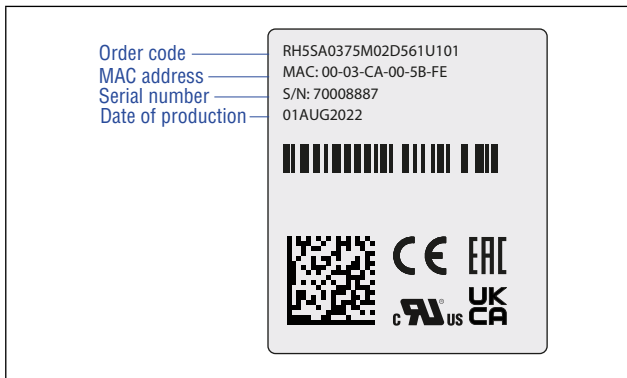
Fig. 1: Example of nameplate of R-Series V RH5 sensor with EtherCAT® output
