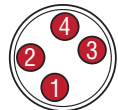
Input voltage, male, 4-pin (D54) integral connector pin-out as viewed from the end of the sensor
