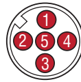
Male, 5-pin (D54) integral connector pin-out as viewed from the end of the sensor
