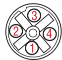
Female, 4-pin (M12-D) Integral connector pin-out as viewed from the end of the sensor
