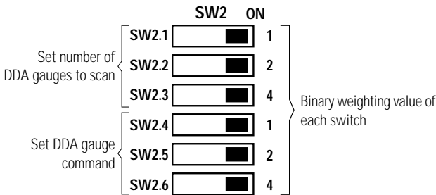
Figure 2.10 DIP Switch #2 Functions (Stand-alone mode)
